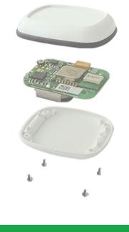
Tag Piccolino is an active mobile locator. Its position and ID is reported within configurable rate. Tracked objects need to be equipped with this device.
